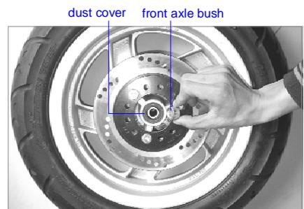
Turn bearing inner race to inspect sliding.
